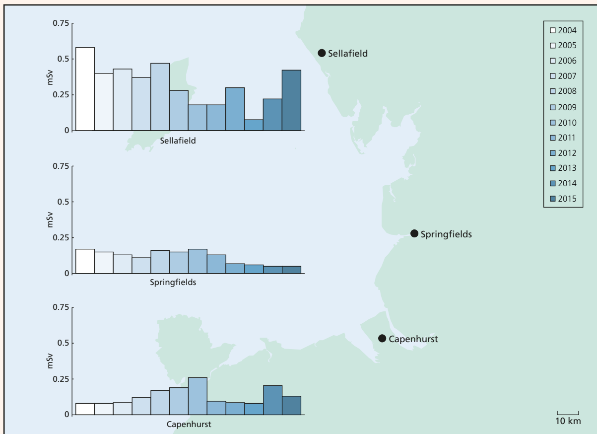
Figure 2.1. Total dose at nuclear fuel production and reprocessing sites, 2004-2015 (Exposures at Sellafield/Whitehale/LLWR receive a significant contribution to the dose from technologically enhanced naturally occurring radionuclides from previous non-nuclear industrial operations)
