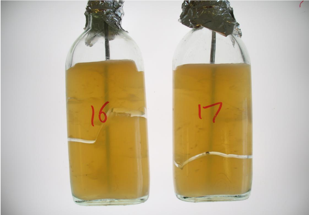
Plate 4 Probes in Disinfectant Hot Water
