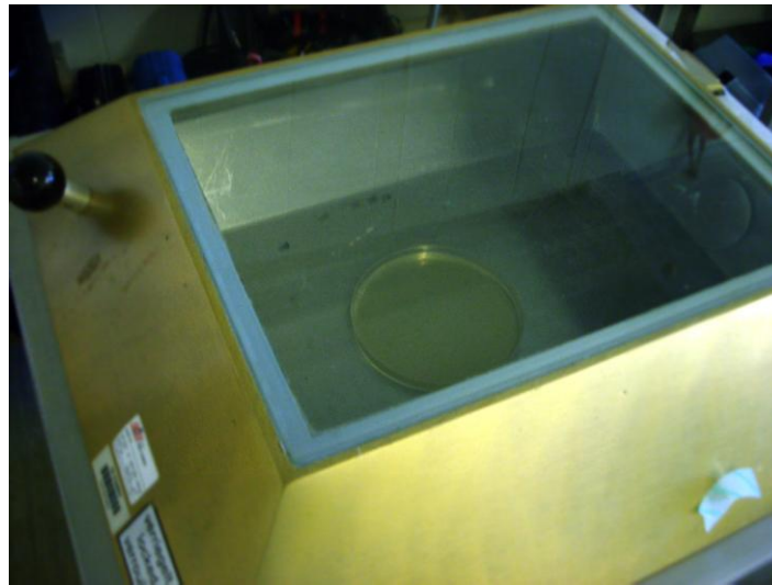
Figure 2: Open control plate test carried out in duplicate before and after packing 300 agar discs contained in vacuum pouches.
