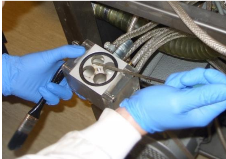
Figure 2: Inoculation of the suction pipe manifold
