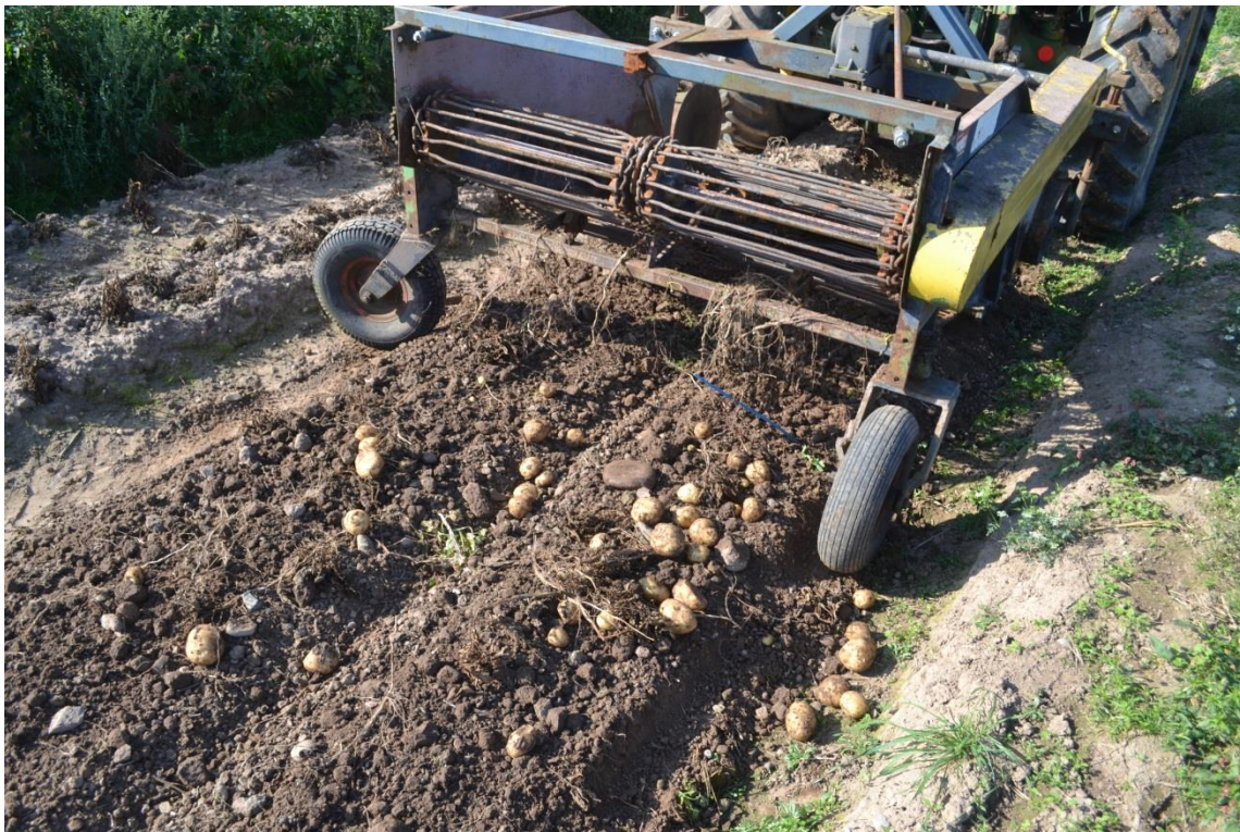
Figure 9 Potatoes were harvested mechanically using a tractor-pulled potato harvester
