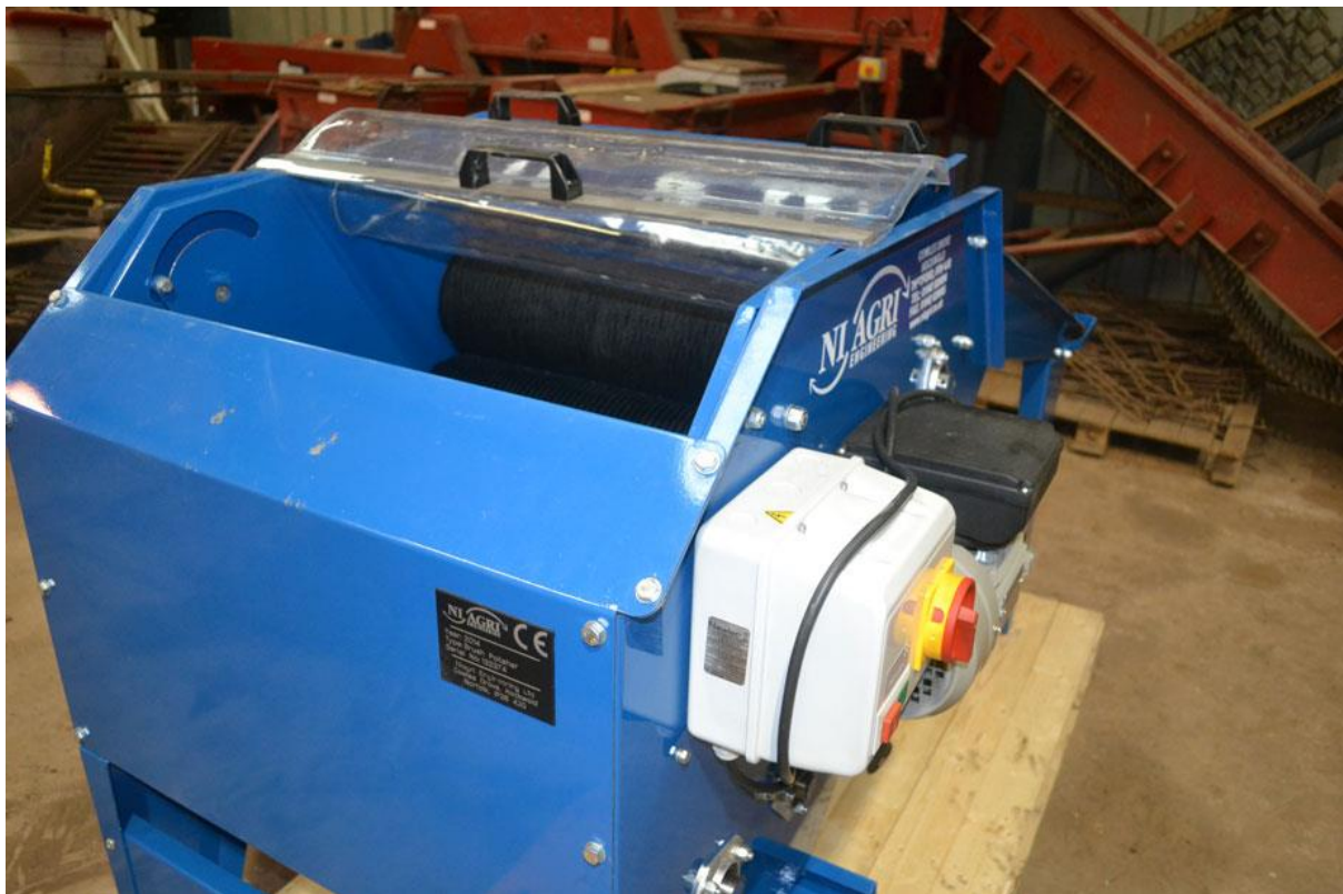
Figure 12 A pilot-scale abrasive brush washer was used to clean carrots in 25kg batches and remove the outer surface of the crop
