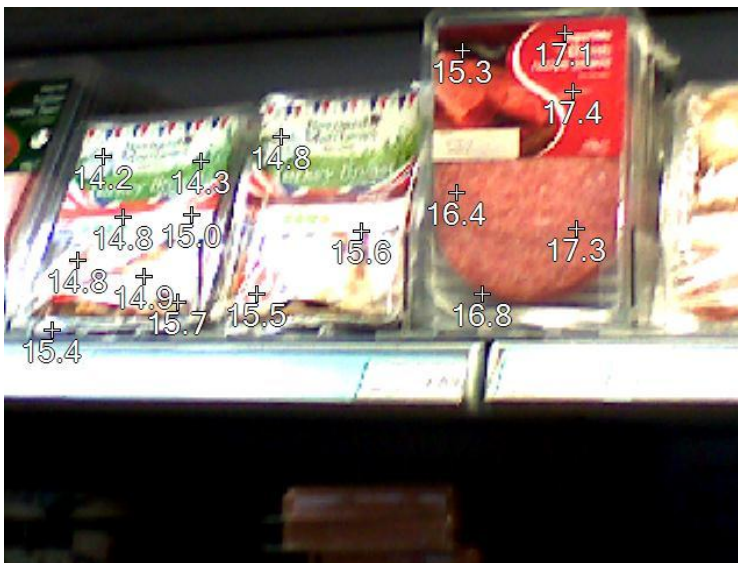
Fig 12b. Spot temperature distribution across several products showing how elevated temperatures are not restricted to just a few samples. The trend for recessed product to be cooler can also be seen.
