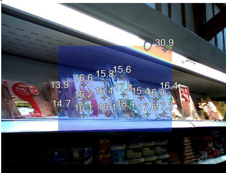
Fig.11b. Spot temperatures in typical chill cabinets showing the relatively high temperature of the illumination strip, over 30°C in both cases.
