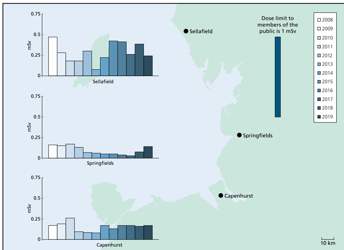
Figure 2.1. Total dose at nuclear fuel production and reprocessing sites, 2008-2019 (Exposures at Sellafield/Whitehaven/LLWR receive a significant contribution to the dose from technologically enhanced naturally occurring radionuclides from previous non-nuclear industrial operations)
