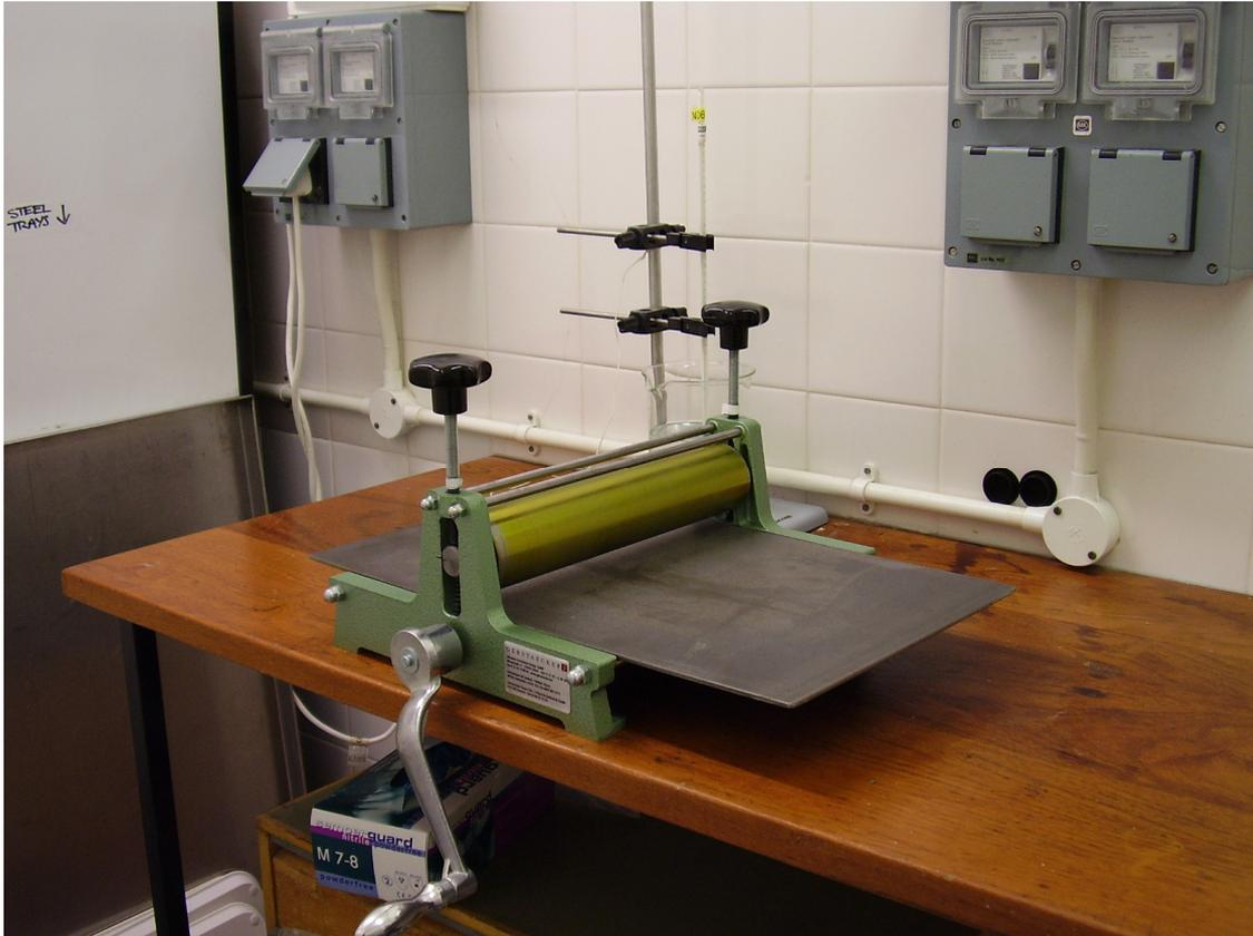
Figure 4. Roll-type printing press employed to flatten fillets of herring and mackerel for worm visualisation.
