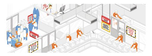
Packaging should be removed and/or destroyed at the end of a production run, including any packaging that may be within the wrapping machine. This is to avoid packaging mix-ups when the product is changed.
